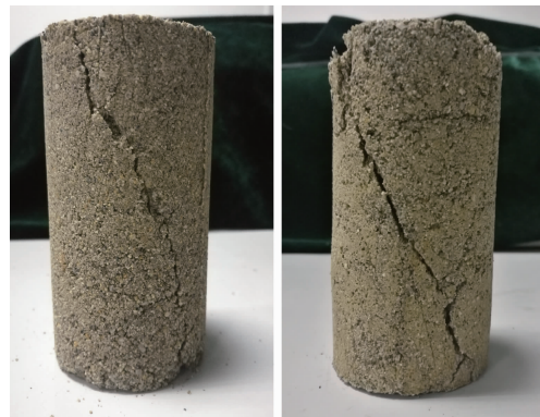
图4 纳米硅浓度20%和改性剂0.2%加固试样破坏特征 Fig. 4 Destruction characteristics of the reinforced samples with nano-silicon concentration of 20% and modifier of 0.2%
