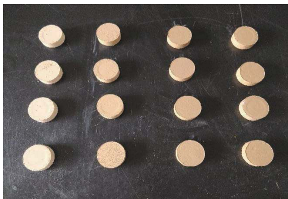
图 1 尖山营膨胀土标准环刀试样 Fig. 1 Standard ring cutter sample of the Jianshanying expansive soil
