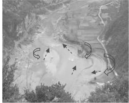
图3 大理石厂回水沱水平环流示意图 Fig.3 The sketch map of the level of circulation at marble factory
